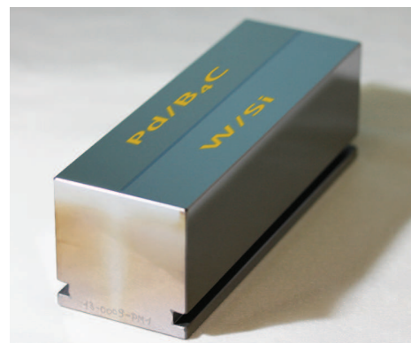
2-stripe multilayer monochromator with harmonic suppression working between 6 keV and 15 keV.
