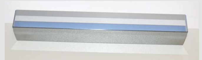
3-stripe multilayer monochromator for applications at synchrotron beamlines between 5 keV and 80 keV.
