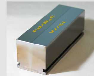
2-stripe multilayer monochromator with harmonic suppression working between 6 and 15 keV.
