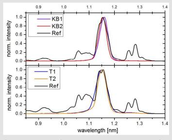
Spectrum emitted from a laser plasma source (LPS) before ("Ref") and after reflection from different multilayer mirrors such as a 1-dimensonally focussing mirrors in a KB arrangement and single toroid segments.
