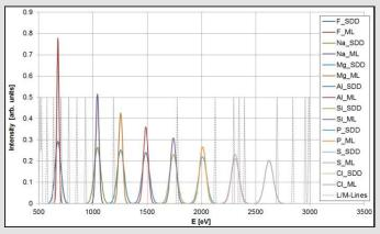
Calculated energy resolution for silicon drift detectors (SDDs) and multilayers for K emission lines from F to CI. Several L- and M-lines of heavier elements are shown, too.
