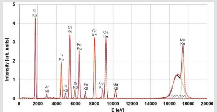
Energy spectra of a 6-element reference sample RF (top) and RG (bottom) measured with a lab TXRF using Mo-K radiation (50 kV excitation). The energy range is covered with peaks of comparable intensity. (*Ga signal from the internal TXRF standard.*)
