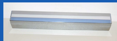
3-stripes multilayer monochromator with Pd/B 4 C (blue), Ir (light grey), Ni/C (dark grey).
