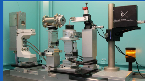
Fig 4: Demonstrator setup – \mu Focus Cu X-ray source, ASTIX-f mirror, object, MLL, X-ray detector
