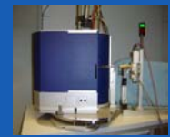
STOE powder diffraction system LaB 6 powder sample / capillary ∅ 250 µm time: 3 min / image plate detector
