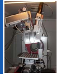
experimental setup: Diffractometer XRD 3003 (Gö-11) for samples up to 200 mm × 200 mm or 8" ∅ and for measurements up to 2θ = 160°
